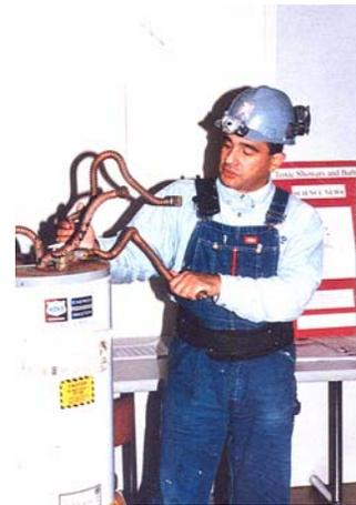
**Ken Russo points out the chloramine corrosion on water heater plumbing.**
